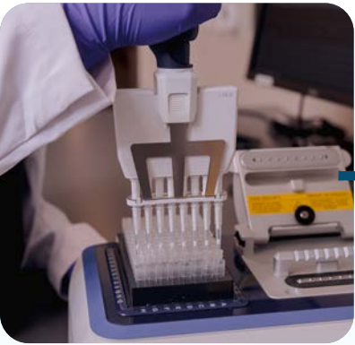
DNA quantity is measured as a quality control using the NanoDrop Eight Spectrophotometer
